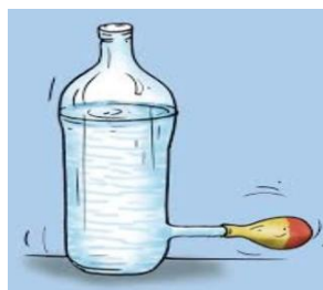
Liquid exert pressure on the wall of the container
